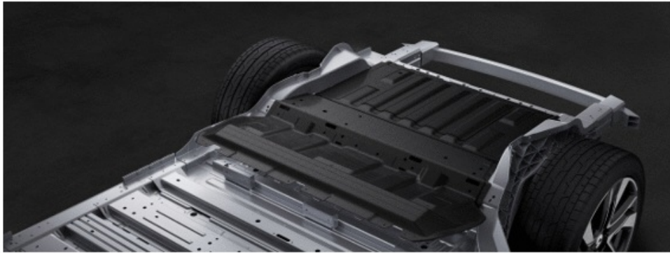
Aluminum alloy and carbon fiber compose the vehicle body
